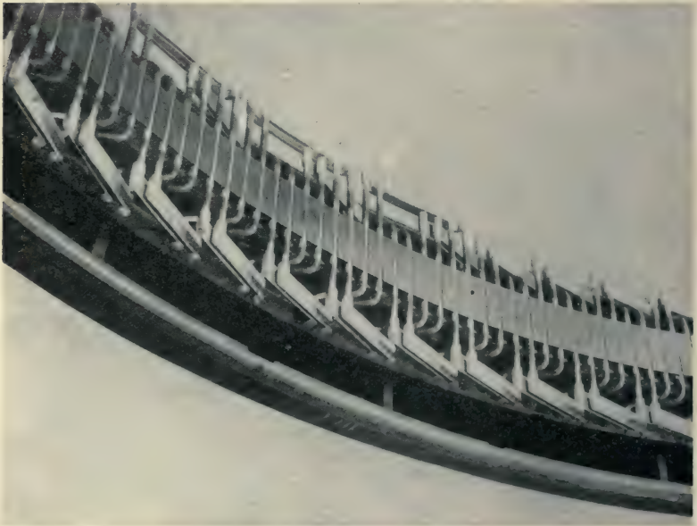
FIG. 270.—Three-phase, Two-slot Wave Winding.
